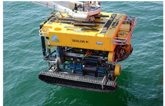
*Underwater cable-laying tractor built by SMD.*
