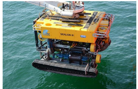
Underwater cable-laying tractor built by SMD.
