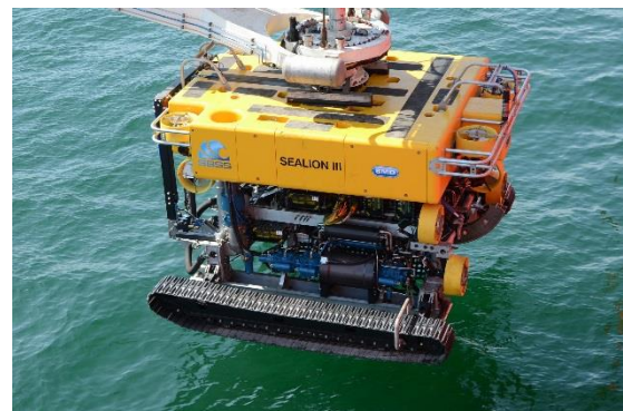
Underwater cable-laying tractor built by SMD.
