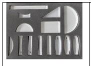
A boxed set of different shaped and sized prisms. Use with LED light source devices to investigate how lenses and prisms change light.
