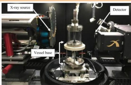
Figure 3 Test vessel inside X-ray scanner
