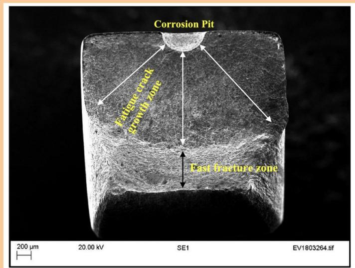
Figure 1 SEM image of an ordinary fractured specimen, experiment on in the sour environment.
