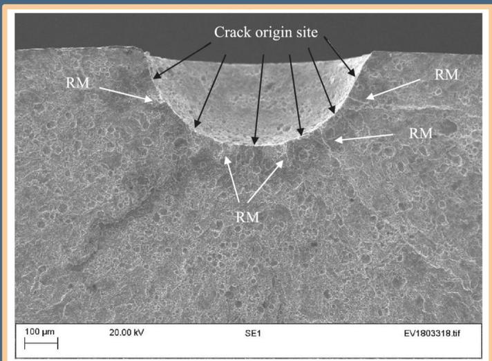
Figure 2 SEM image demonstrating ratchet marks and crack origins on a specimen with an applied stress amplitude of 185 MPa.
