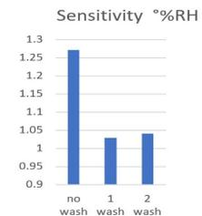
Washing has the potential to reduce the sensitivity of the sensors and even stop them working all together. After 1 wash in this test the sensitivity dropped dramatically but this doesn't occur after the 2nd wash. This is because the fabric is treated with an antibacterial spray after manufacture which is washed off after the first wash.
