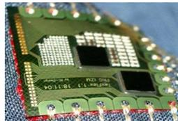
Embedding electronic sensors in the material instead of simply attaching conventional electronics to its surface, has many advantages including reduced mass and increased comfort.
