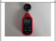
Digital anemometer. This portable anemometer is a practical measuring meter which can measure wind speed and temperature. It also has wind scale and windchill indication.
