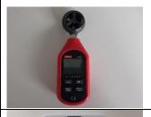
Digital anemometer. This portable anemometer is a practical measuring meter which can measure wind speed and temperature. It also has wind scale and windchill indication.
