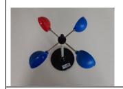
Spinning wheel anemometer. The stronger the wind blows, the faster the wheel rotates. The anemometer counts the number of rotations, which is used to calculate wind speed.
