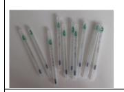
10 thermometers for taking the air temperature with a range of -10 to +50 degrees. Each degree is marked with every 10 degrees labelled.
